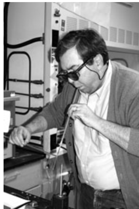
Above: Dr. Sidebottom is seen glass working: making quartz ampules for spectroscopy.
